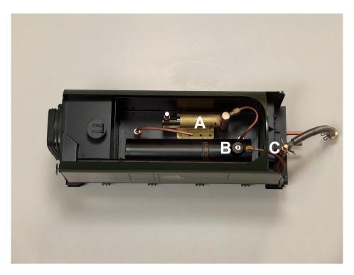
**A:** Hand pump. **B:** Gas tank filler valve. **C:** Gas control valve.
