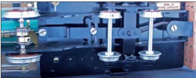
Left: The mounting for the rear truck and coupling is not an elegant method of control. Articulated and protruding through the buffer beam, the coupler sits so close that it appears fixed.
