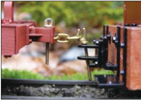
Above: Someone at Accucraft clearly thought the loco would spend its life in a glass case! The difference in coupler height is very marked here with rolling stock from the same maker. The LB&HT cure uses pins from Brandbright's RSA68 coupler, chain from the local hardware store and thought from yours truly...
