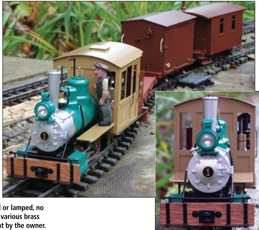
Above: Someone at Accucraft clearly thought the loco would spend its life in a glass case! The difference in coupler height is very marked here with rolling stock from the same maker. The LB&HT cure uses pins from Brandbright's RSA68 coupler, chain from the local hardware store and thought from yours truly...
